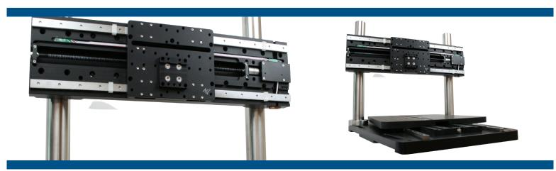
GTS-Series Gantry Translation Stages offer three precision closed-loop DC servo motor linear actuators available in a range of travels. The standard 15-inch unit, shown, allows 380 mm of travel in the X- and Y-coordinates and 100 mm (4") of travel in the Z-axis, with smaller and larger travel ranges available. An optional fourth axis controls the zooming video microscope, shown, available with zoom ranges as high as 16X.
