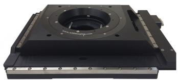
The PRS-1000 Precision Rotary Stage utilizes ASI's proven precise control through the use of closed-loop DC servomotors and angle encoded out drive. The low profile design with the ability to be integrated into our MS-2000 XY stages offers flexible usage. Standard versions have a Ø 95 mm clear through aperture, use all of ASI's C size inserts, and have M3 tapped holes on 125 mm D.B.C. The PRS-1000 is also available with solid top plates for vacuum applications and M6 on 25mm centers.
