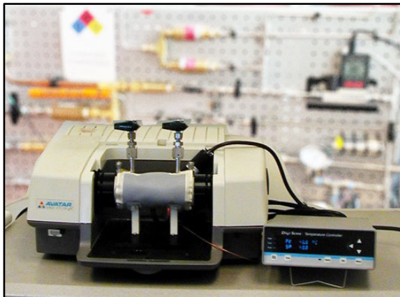
10cm complete with heater and purge hardware mounted in the FTIR
